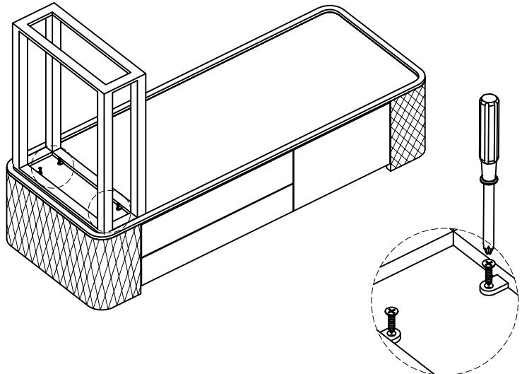
2.Place the glass on the table and move the dresser to the side without hardware feet for bottom support
