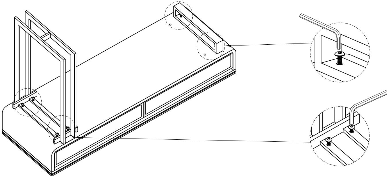
2. The mobile dressing cabinet can be placed on the support rack under the dressing table
