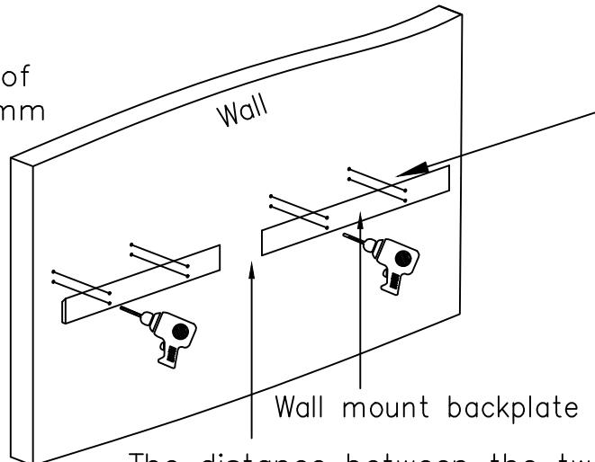
ensure that the two boards are aligned properly.
