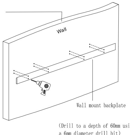
2. After the drilling is completed, insert the expansion plug into the wall hole, place the wall-mounted backboard, and insert the self-tapping screw into the position where the wall hole connects to the backboard hole. Tighten the screw with a screwdriver.
