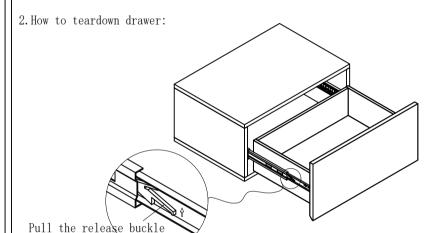
Open the drawer as far as possible. Pull the disassembly buckle upwards, while pull another disassembly buckle downwards. Separate the drawer from the guide rail.
