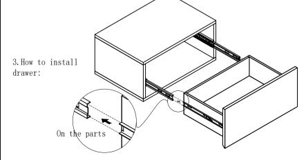
1. Align the two guide rail parts of the drawer, and then push the drawer forward to the bottom
