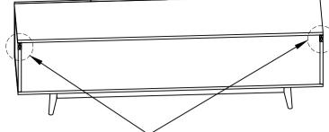
(1) Place the Anti -tipping (2) Use a marked pen label the device on the back of the side location of the level of the cabinet plate of the cabinet.
