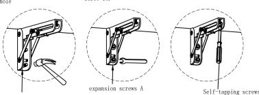
(Drill to a depth of 60mm using a 10mm diameter drill
