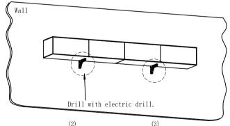
Hammer the expansion screws B into drilled hole
