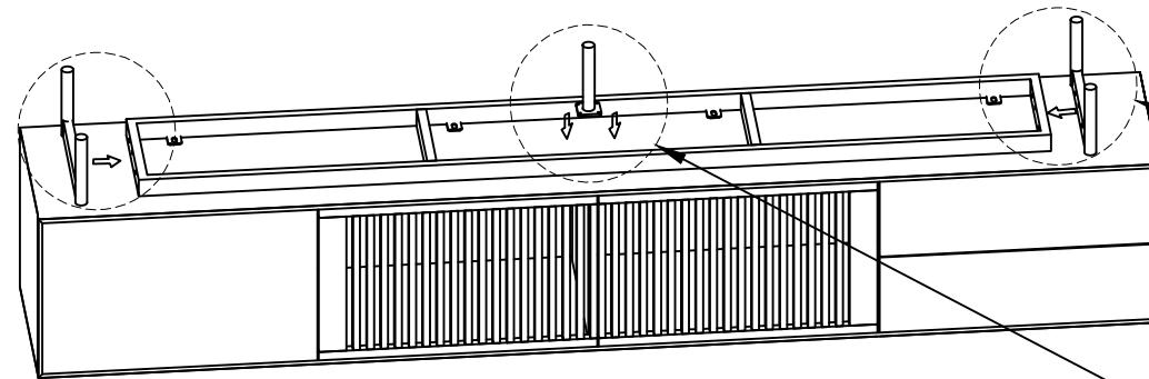
(1.1) Place the side feet on both sides of the foot stand to align the holes, and then insert the hexagonal socket thread and gasket into the foot stand and tighten them with a wrench
