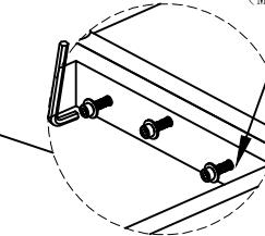
(1.2) Place the middle foot in the center of the cabinet bottom plate, and use a screwdriver or electric drill to drive in the tapping screw
