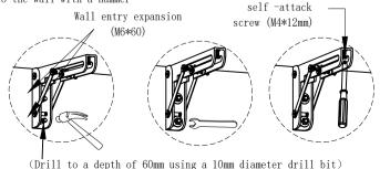
(3) Tighten the self -attack screw with a screwdriver
