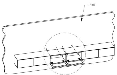
(1) After marking the position with a marking pen, use an electric drill to drill holes in the wall
