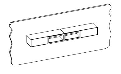
1. Place the cabinet at the required height, and mark the holes and walls in the cabinet with a marker pen.
