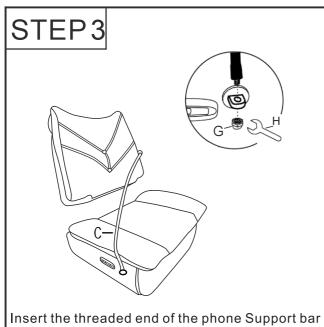
(Part C) into the metal hole on the right side of the seat(Part B), then tighten it with the nut (Part G) under the hole.
