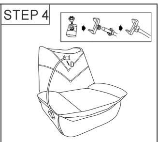
Screw down the Plastic nut from the Mobile phone holder (Part D), cross the Plastic nut to the Phone support bar (Part C), then insert the Phone holder (Part D) to the support bar (Part C), tighten screw the plastic nut.
