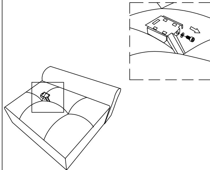
3. Insert the fasteners at the bottom of the sofa backrest into the seat cushion support frame, then tighten them with screws as shown in the figure
