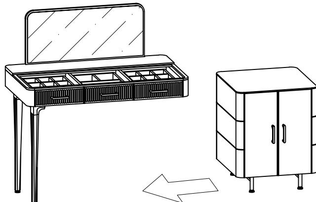
2. Position the vanity mirror on the corresponding location on the backboard of the dressing table, align the holes, insert the screws, and tighten them with a wrench.
