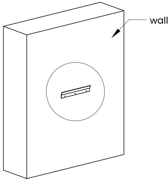
(1) Place the vanity mirror wall plate at the appropriate height on the wall, mark the location with a marker, and drill the holes with an electric drill.
