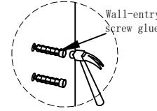
(5) Place anti tipping on the wall and use an electric drill to drive the self tapping screws into the wall
