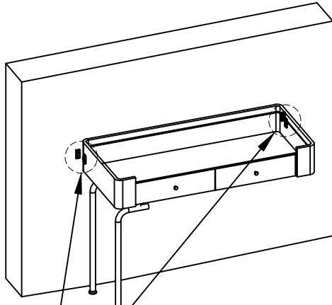
(1) The anti tipping device is installed on the cabinet side panel
