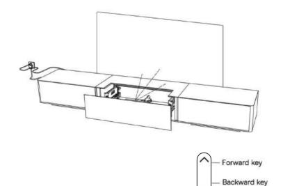
Use the front/back buttons to adjust the cabinet extension until the projection is clear. Hold for 10 seconds to save position (auto-memorized for next startup).
