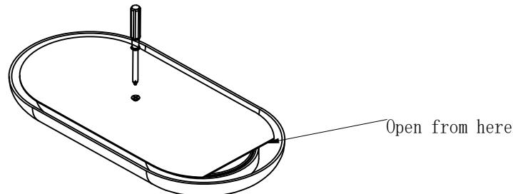
3. The button cell is placed in the groove with the positive pole side down (Smooth flat side downwards)
