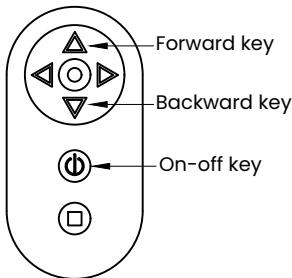
3. Use the forward and backward keys on the remote control to adjust the distance of the cabinet, then place the projector inside. (After adjusting the position of the cabinet, let it stand for 30 seconds to complete the position setting, and press the on-off key to retract)
