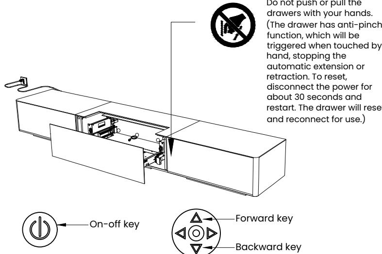
Do not push or pull the drawers with your hands. (The drawer has anti-pinch function, which will be triggered when touched by hand, stopping the automatic extension or retraction. To reset, disconnect the power for about 30 seconds and restart. The drawer will reset and reconnect for use.)
