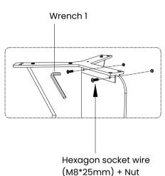
4. Align the connection holes on the bottom and top of the desktop with the connection plate and tighten with an Allen key.
