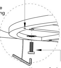
Hexagon Socket Machine Screws(M8\*30mm)+Gasket
