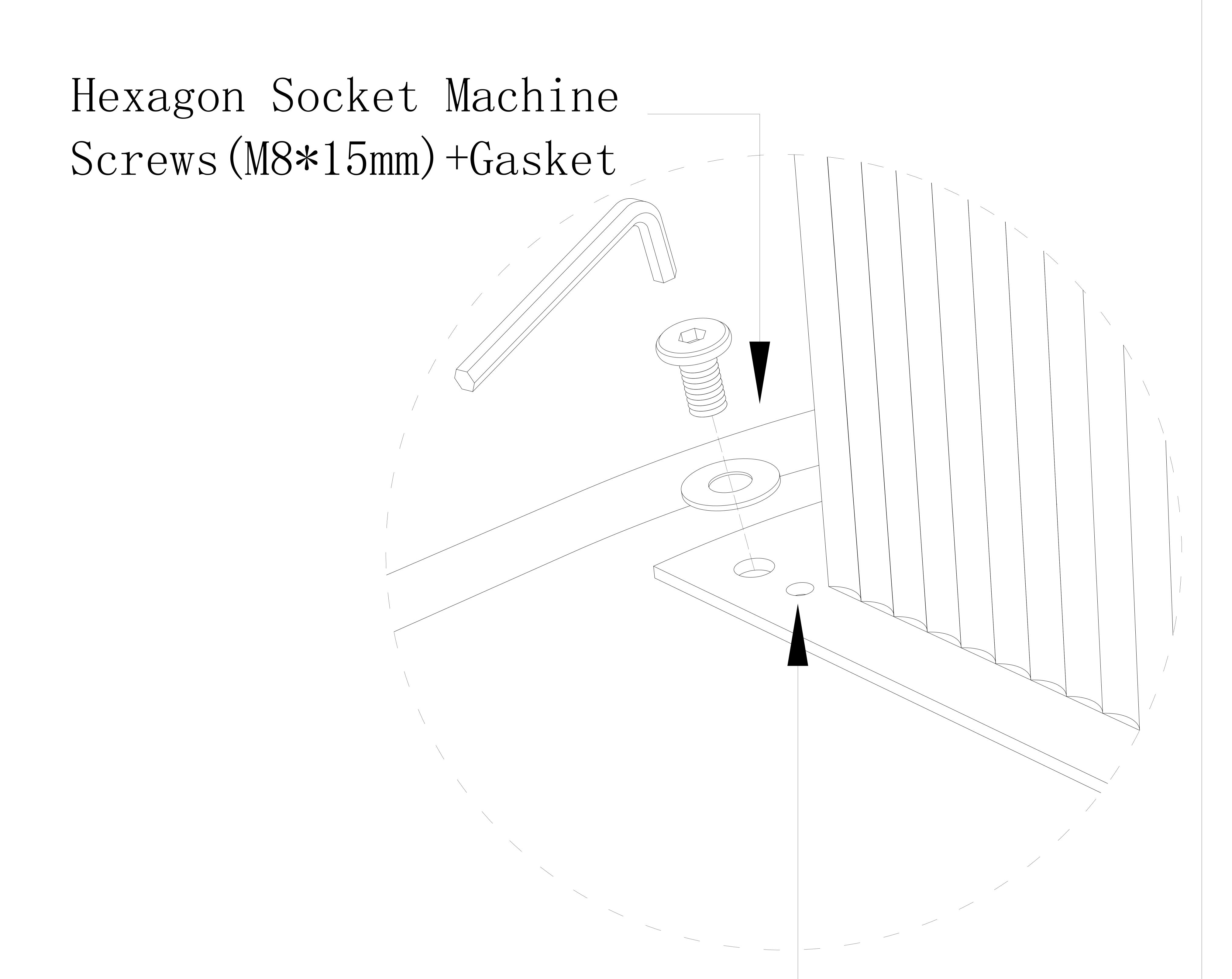
Spare Holes (Hexagon socket machine screws holes can be screwed into the use of Self-drilling screw when damaged)
