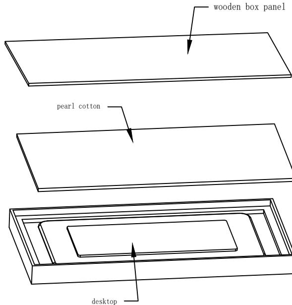
3. Place the desktop on the removed pearl cotton place (avoid collision and damage to the desktop).
