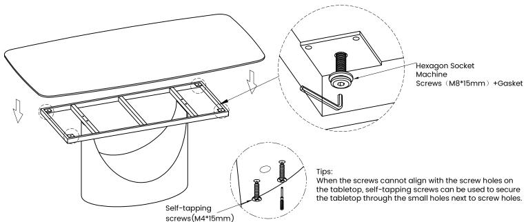
4. Installation Completed (If the product is unstable or wobbles, please adjust the adjustable feet at the bottom of the product to ensure it is level with the ground.)
