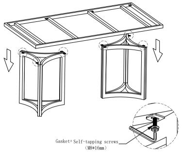
2. Place the desktop above the support frame, put the self-tapping screws in the ear piece position, and tighten the screws with a screwdriver.
