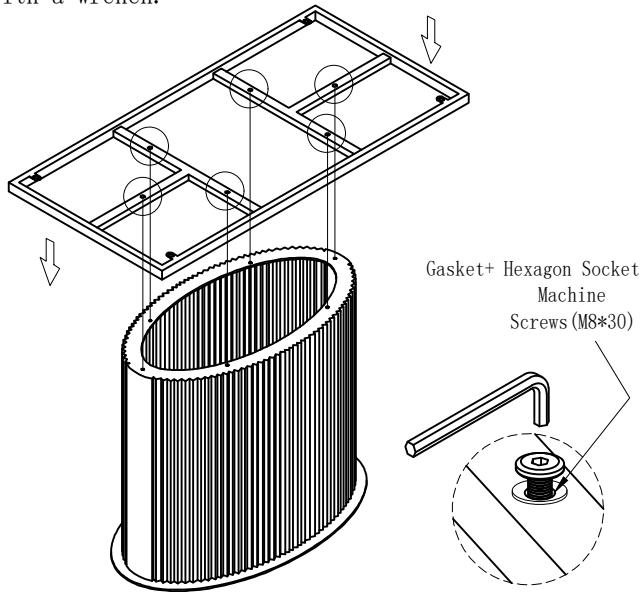
2. Place the table top on top of the frame, put in the hexagon socket machine screws and gasket, and tighten the hexagon socket machine screws with a wrench.
