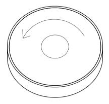
3. The button cell is placed in the groove with the positive pole side up (Smooth flat side facing up)
