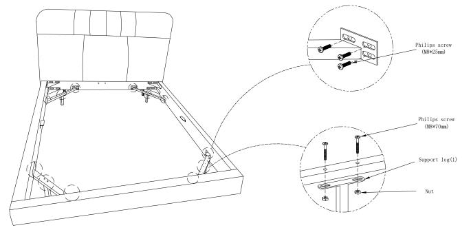
4. Install three support legs(2) on the long rod and install the long rod to the corresponding hole position
