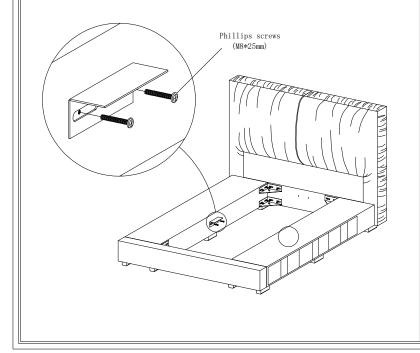
4. Install the intermediate load-bearing support frame
