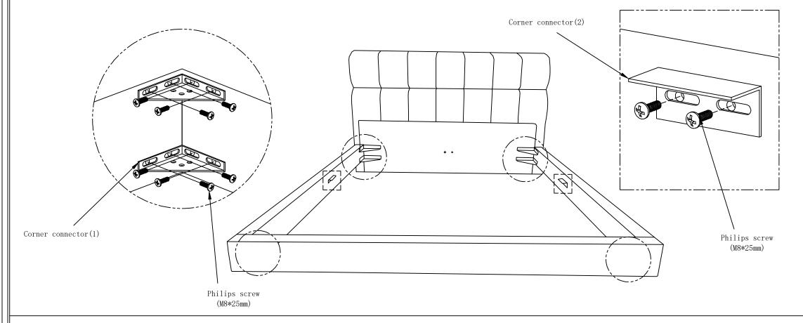
2. Install the support legs (1) at the long corner connector (Paste a non-slip gasket on the bottom of the support leg)
